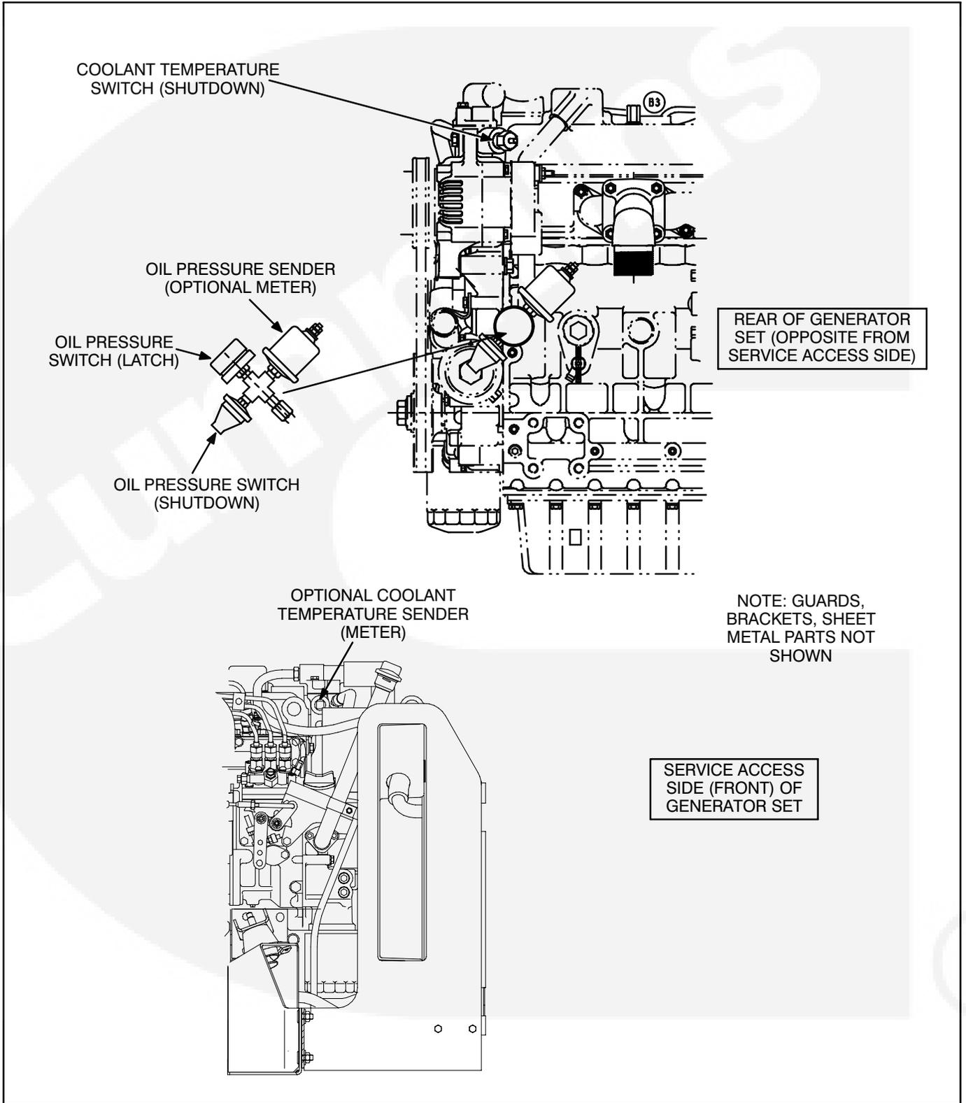
**FIGURE 13. OIL AND COOLANT SENSOR LOCATIONS**
